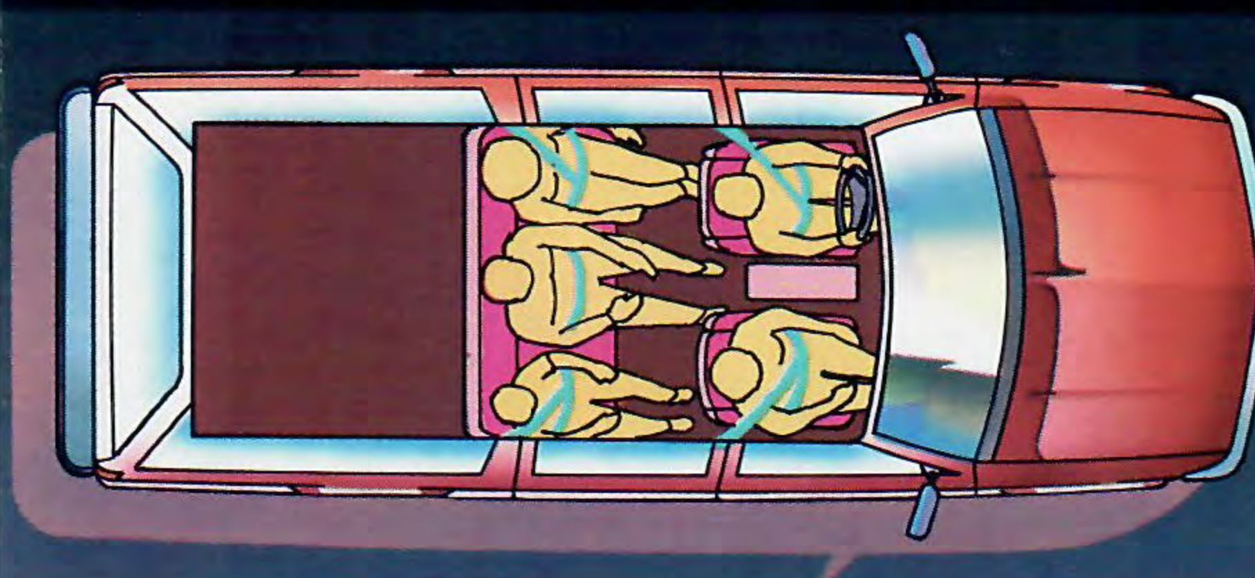
B 5-passenger, with available two front high back buckets and center 3-passenger bench.
